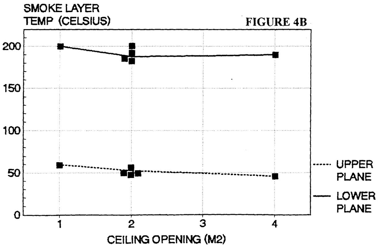
Figure 4A-B. Measured smoke-free height and average smoke layer temperature. Fuel size is 0.56 m<sup>2</sup>. Opening between planes is 0.5 m<sup>2</sup>.
