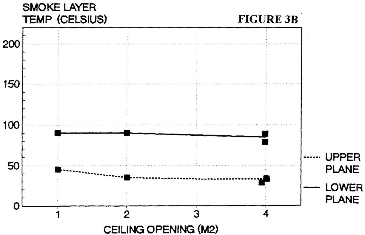
Figure 3A-B. Measured smoke-free height and average smoke layer temperature. Fuel size is 0.25 m<sup>2</sup>. Opening between planes is 1.0 m<sup>2</sup>.
