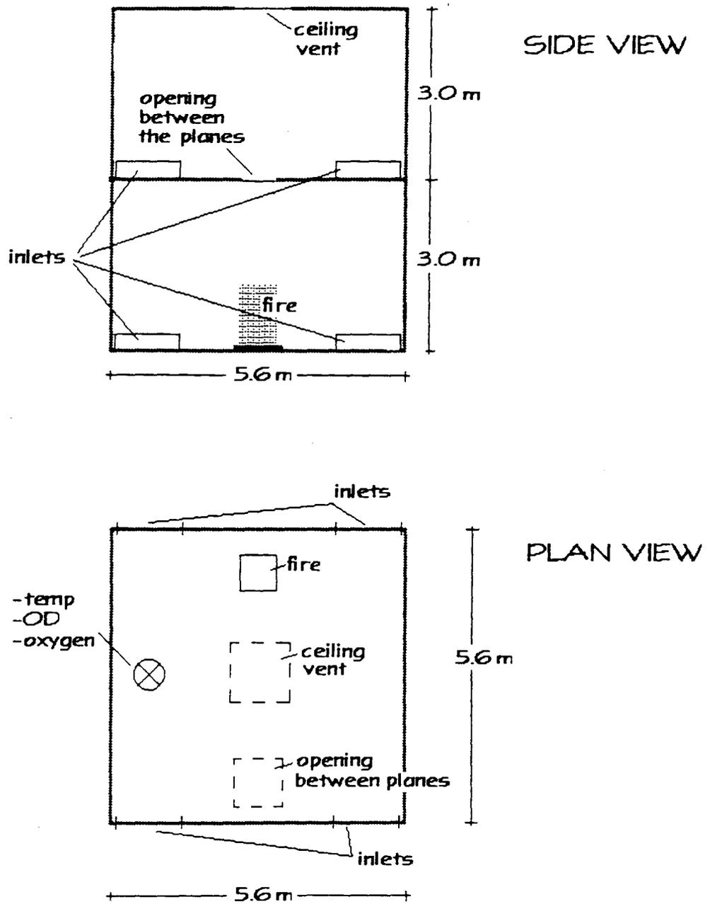
Figure 1. Test geometry and instrumentation.
