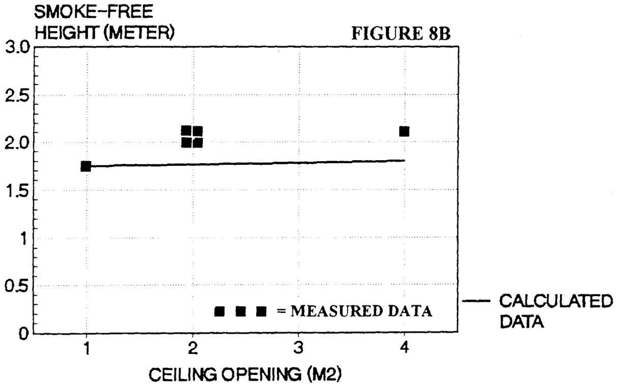
Figure 8A-B. Calculated data by CFD model are compared with measured data. The quantity compared is the smoke-free height.
