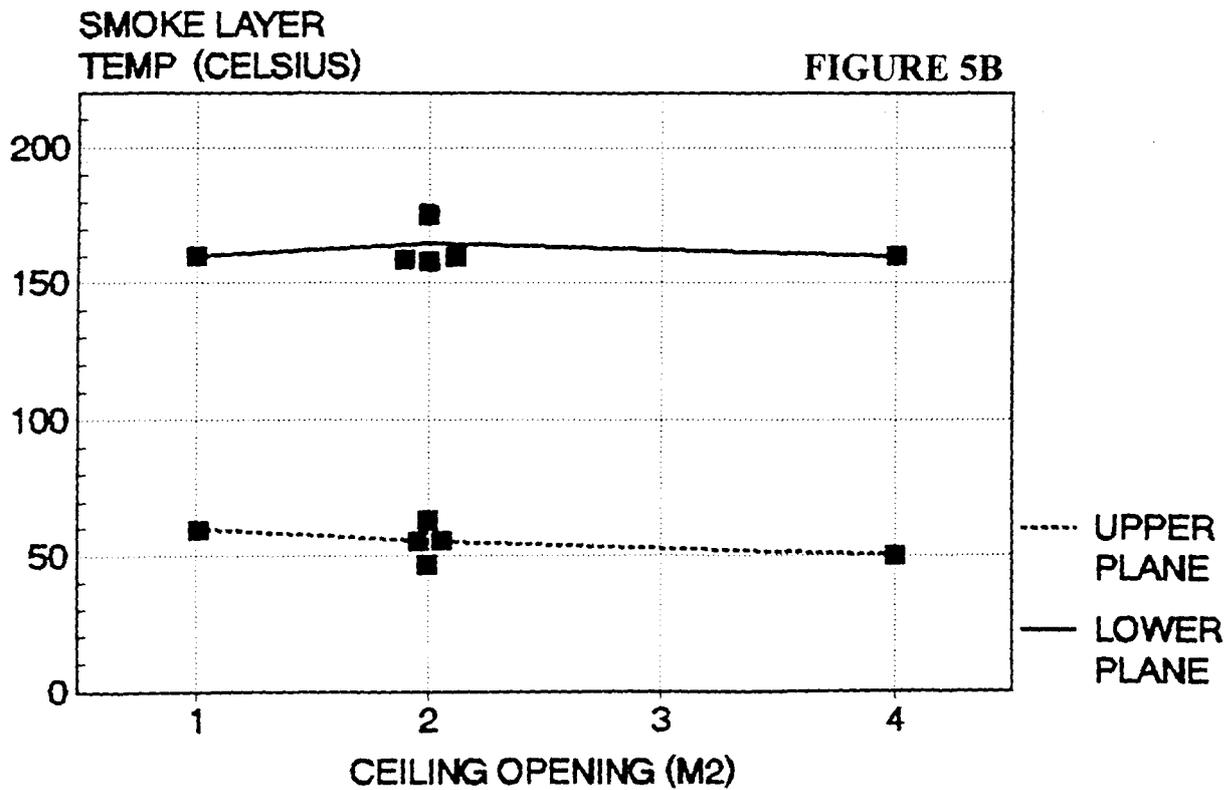
Figure 5A-B. Measured smoke-free height and average smoke layer temperature. Fuel size is 0.56 m<sup>2</sup>. Opening between planes is 1.0 m<sup>2</sup>.
