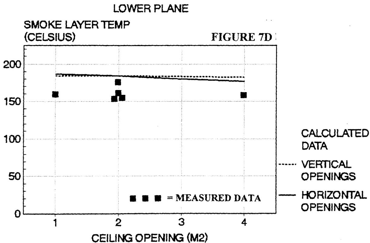
Figure 7A-D. Calculated data by zone model are compared with measured data. The quantities compared are the smoke-free height and average smoke layer temperature.
