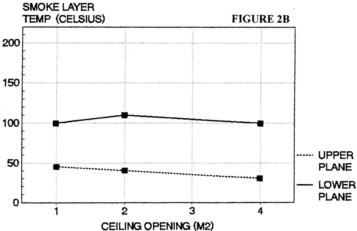
Figure 2A-B. Measured smoke-free height and average smoke layer temperature. Fuel size is 0.25 m<sup>2</sup>. Opening between planes is 0.5 m<sup>2</sup>.
