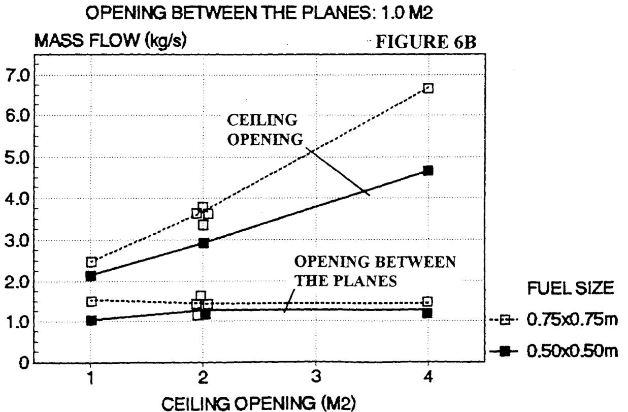
Figure 6A-B. Calculated mass flow values through horizontal openings based on velocity values measured centrally at the openings. The flow coefficient is assumed to be 0.6.
