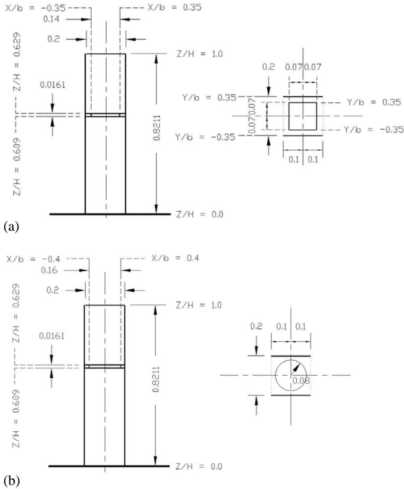
**FIGURE 1.** High-rise building models: (a) A large square-planned main services core at the centre of the refuge floor, and (b) A large circular based main service core at the centre of the refuge floor
