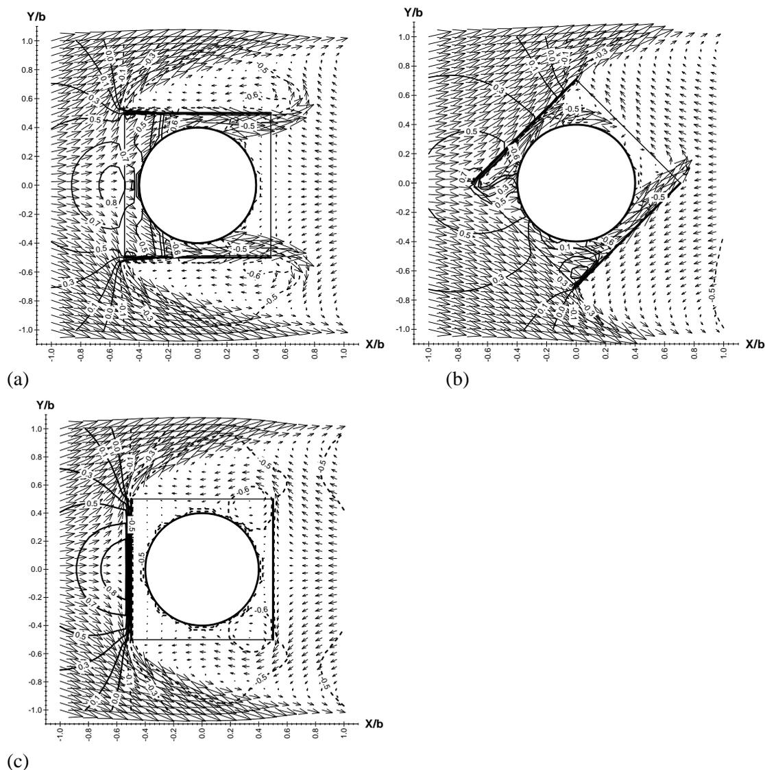
**FIGURE 3.** Normalised velocity vector distribution and contour line of pressure coefficient over the symmetry horizontal flow plane of the refuge floor which is located at the building mid-height with a large circular-based main services core located at its centre: (a) Wind blowing at normal incident to the building (stream-wise), (b) Wind blowing at an angle diagonally to the building, and (c) Wind blowing at an angle perpendicular to the solid side walls of the refuge floor
