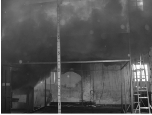
(a) Smoke layer remained stable
