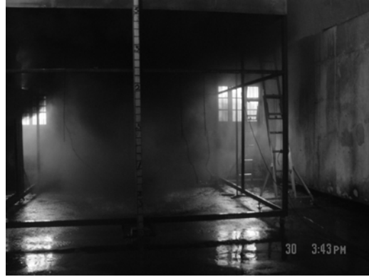
(c) Smoke reaching the floor
