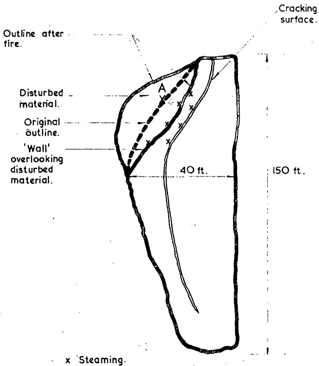
FIG. I. PLAN OF SLUDGE HEAP.
