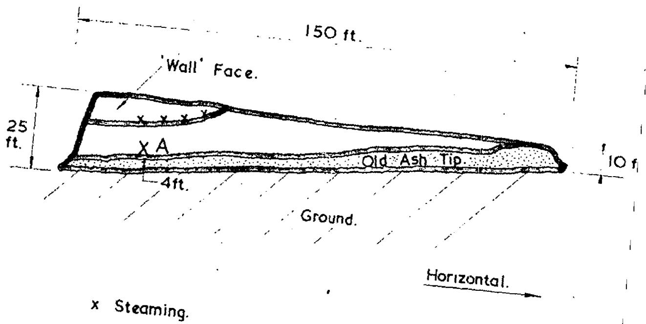
FIG. 2. SECTION OF SLUDGE HEAP
