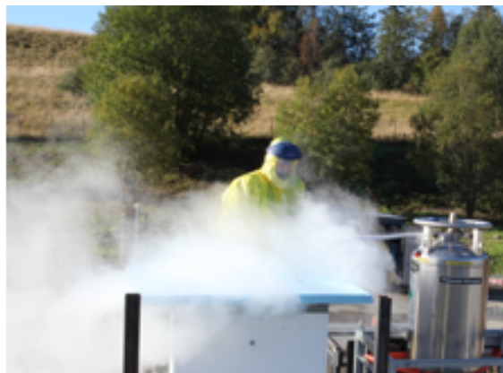
Filling of liquid nitrogen. 250 liters of liquid nitrogen are poured into the upper part of the test rig before this is released upon the test specimen mounted below. Photo: Reidar Stølen, SP Fire Research.
