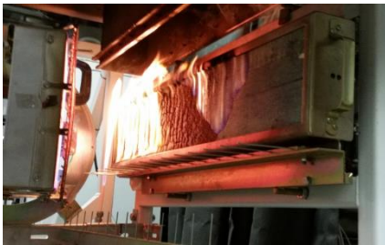
Figure 2 We have been studying the effect of Adhesive breakdown in Engineered Timber. Results appear at the Fire and Materials conference.
