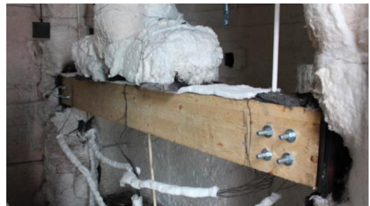
Figure 3 Timber Connection Furnace Tests were also presented at the Fire and Materials Conference
