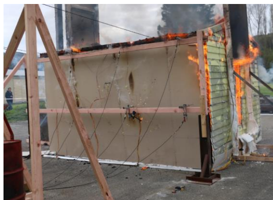
Figure 1. Full-scale horizontal fire spread experiment with lateral loading
