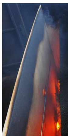
EPS burning slowly in the gap between a wooden fiberboard and concrete wall. Not until all the EPS was burnt to the bottom, the wood started to burn vigorously.
