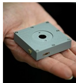
Miniaturized particulate sensor (photo by Paul Greenberg, NASA)
