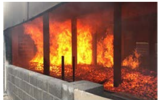
Figure 1. Traveling fire tests with different openings and gas temperatures at ceiling levels along the length of compartment
