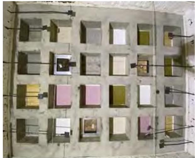
*View of the Pionki Material Survey samples on the ceiling of the furnace*
