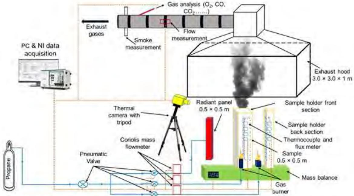
Figure 2: A schematic of new test bench under development at institute Pprime to study thermal decomposition, combustion and flame propagation on ETI setup.
