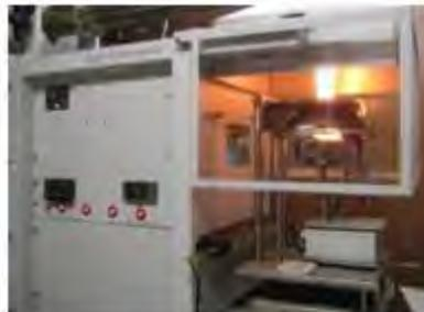
*Reaction-to-fire test using a cone calorimeter.*
