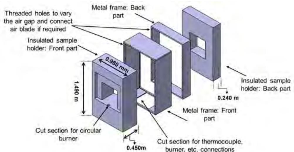
Figure 3: A 3D model of sample holder assembly.
