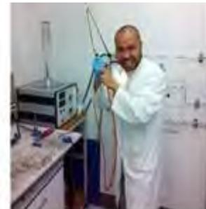
*Flammability test being done by Oisik using limiting oxygen index.*
