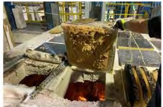
*Charring remains of wood blocks, with visible thermocouples inside (left), a sample of mortar fire protection system after the ISO834 exposure (90 minutes)*
