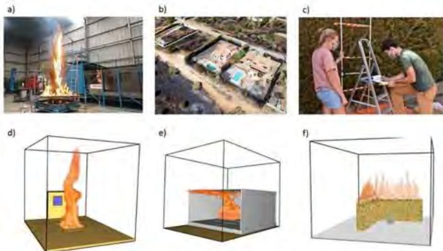
Figure 2. Activities to understand factors and processes at the WUI home-owner level; a) experimental burns at ADAI premises; b) Analysis of WUI accidents; c) Analysis of fuel load in hedgerows; FDS simulations of fire impact in d) glazing systems, e) semi-confined spaces, f) LPG tanks.
