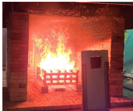
Figure 1: Painted steel surface fire test.
