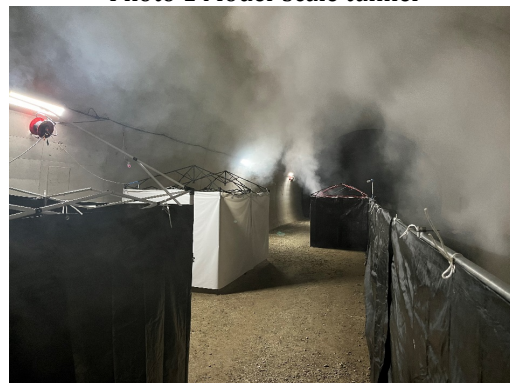
Photo 2 Smoke generation in full-scale tunnel
