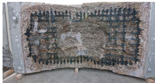
Tunnel Lining Segment after Fire Test
