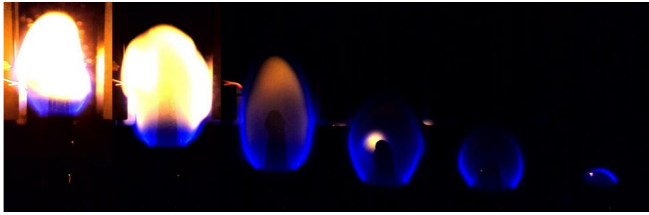
Composite image of a flame spreading in microgravity on the ISS as the oxygen decreases and it moves towards extinction.
