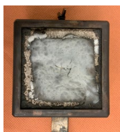
(a) PVC Wallpaper at 20kW/m 2 under air
