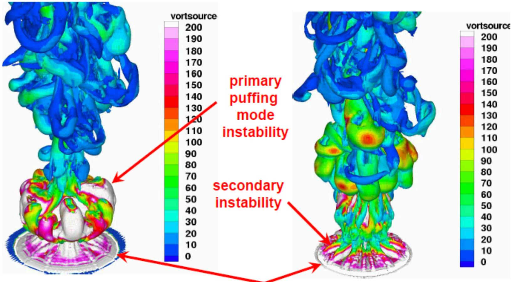
Peak production occurs at base of plume at small scales of motion
