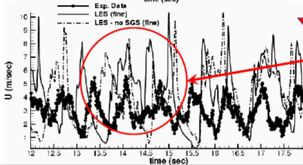
Additional resolution also captures secondary instabilities resulting in a more irregular signal
