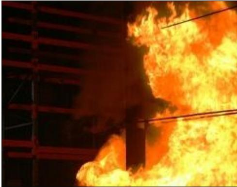
Pool fire test on a steel column at SP
