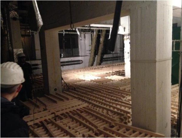
Figure 1: 7 tonnes of wood in one continuous fuel bed
