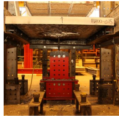
Tested slab-column specimen in The University of Edinburgh laboratory
