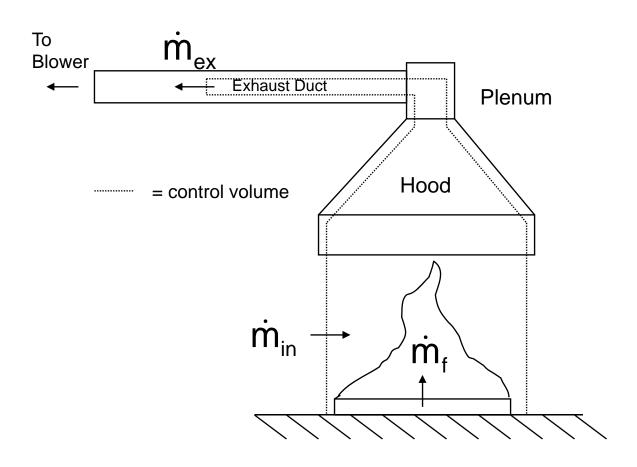
$$\Delta \dot{m}_{\text{O}_2} = \dot{m}_{\text{O}_2,\text{in}} - \dot{m}_{\text{O}_2,\text{ex}}$$
